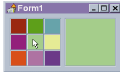
Figure 1: This mini-program sets the color of the panel at right to the color of the panel selected by the user.
